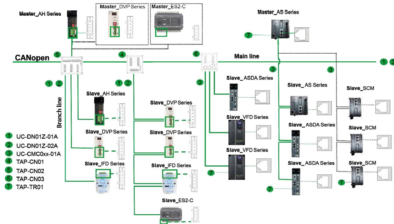
Note: CANopen suggests that users connect a terminator to each end of a CANopen cable to main the stability of signals.
