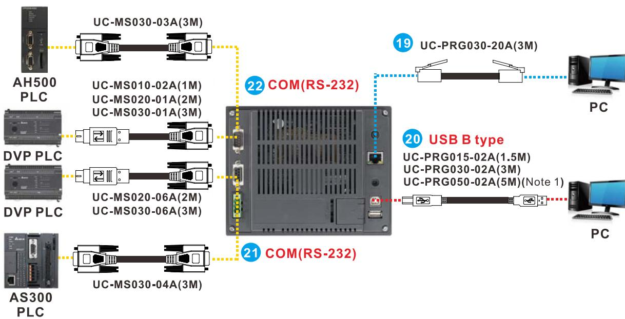
Note1: UC-PRG050-02A is used for transferring input signals between the interface panel and the controller. The cable is used exclusively for all-electric injection molding machines.
