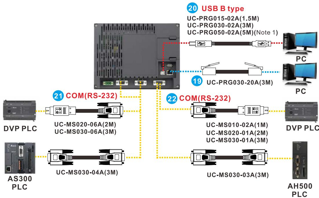
Note1 : UC-PRG050-02A is used for transferring input signals between the interface panel and the controller. The cable is used exclusively for all-electric injection molding machines.
