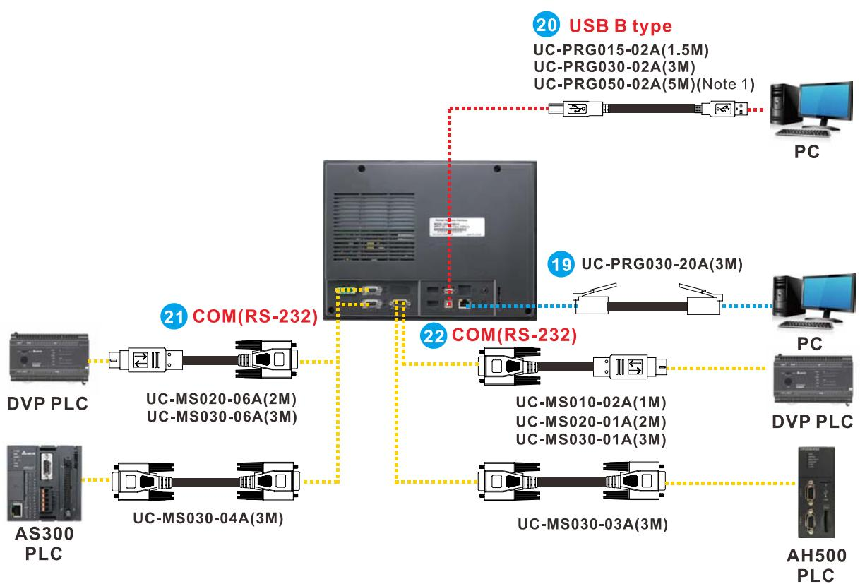
Note1 : UC-PRG050-02A is used for transferring input signals between the interface panel and the controller. The cable is used exclusively for all-electric injection molding machines.
