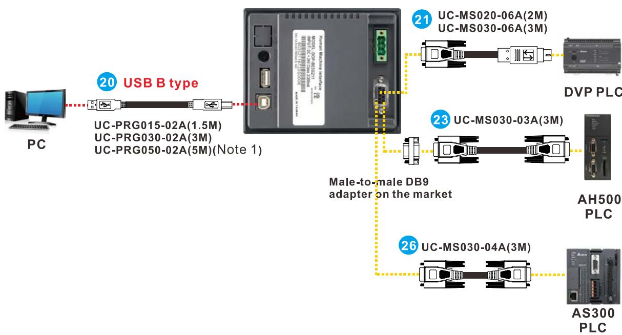
Note1 : UC-PRG050-02A is used for transferring input signals between the interface panel and the controller. The cable is used exclusively for all-electric injection molding machines.
