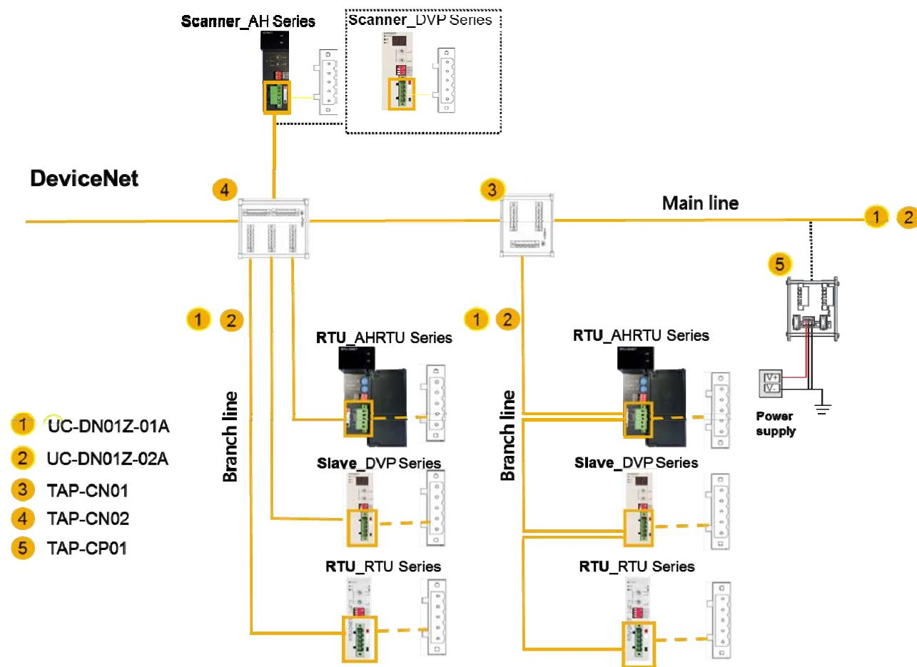
Note: DeviceNet requires that users connect a terminator to each end of a DeviceNet cable. The resistance of the terminators connected is  $121 \Omega$  (1/4 watts). Please refer to section 4.3.3 for more information about a terminator.
