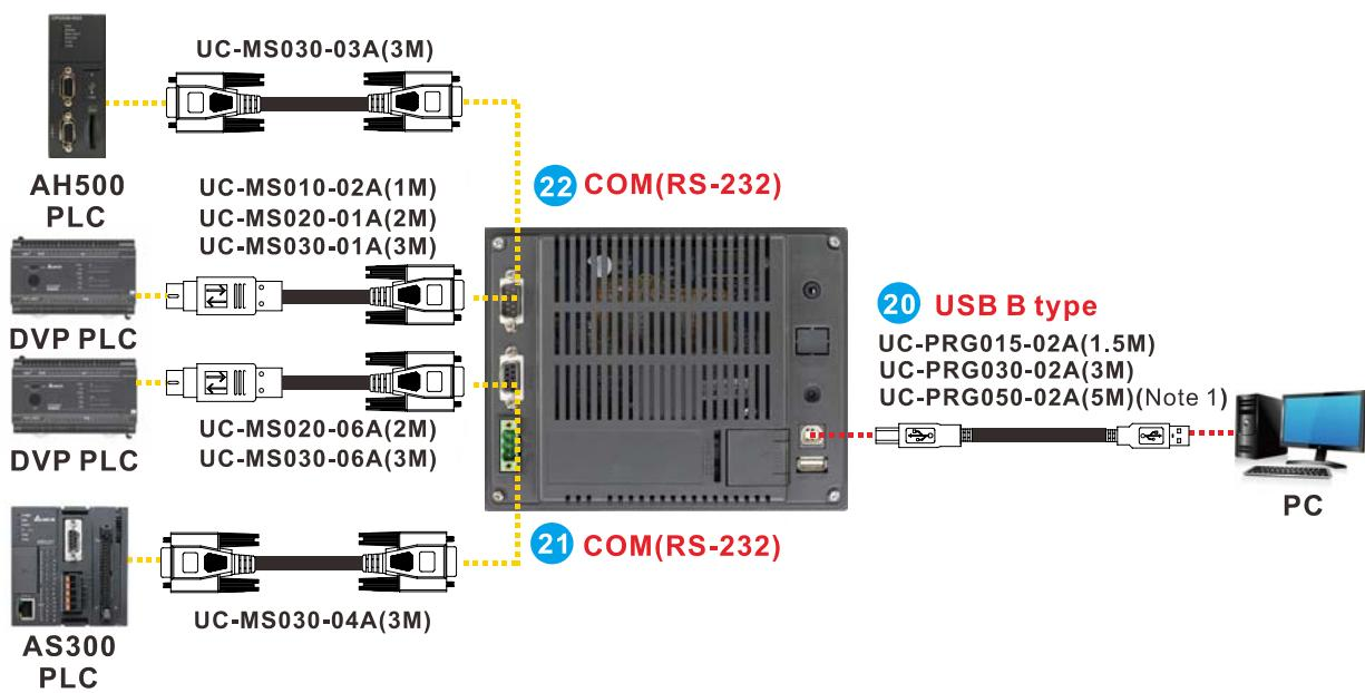
Note1: UC-PRG050-02A is used for transferring input signals between the interface panel and the controller. The cable is used exclusively for all-electric injection molding machines.
